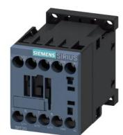
power contactor, AC-3e/AC-3, 9 A, 4 kW / 400 V, 3-pole, 230 V AC, 50/60 Hz, auxiliary contacts: 1 NC, screw terminal, size: S00
