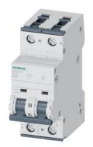
Circuit breaker Universal current 440 V DC 400 V AC 10kA, 2-pole, C, 40 A
