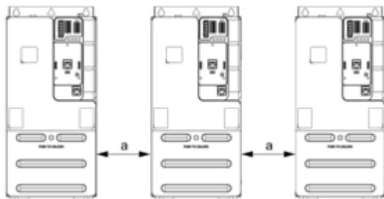
$a \geq 50$  mm (1.97 in.) from 50...60°C, no restriction below 50°C
