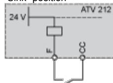
"PLC" position with PLC transistor outputs
