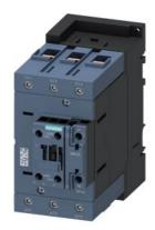
power contactor, AC-3e/AC-3, 80 A, 37 kW / 400 V, 3-pole, 230 V AC, 50 Hz, auxiliary contacts: 1 NO + 1 NC, screw terminal, size: S3  $\,$
