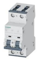
Circuit breaker Universal current 440 V DC 400 V AC 10kA, 2-pole, C, 10 A
