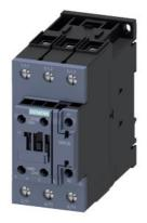
power contactor, AC-3e/AC-3, 80 A, 37 kW / 400 V, 3-pole, 20-33 V AC/DC, 50/60 Hz, with integrated varistor, auxiliary contacts: 1 NO + 1 NC, screw terminal, size: \$2\$
