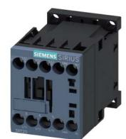
power contactor, AC-3e/AC-3, 16 A, 7.5 kW / 400 V, 3-pole, 110 V AC, 50/60 Hz, auxiliary contacts: 1 NO, screw terminal, size: S00
