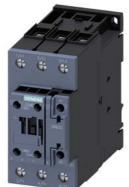
power contactor, AC-3e/AC-3, 41 A, 18.5 kW / 400 V, 3-pole, 110 V AC, 50 Hz, auxiliary contacts: 1 NO + 1 NC, screw terminal, size: S2  $\,$
