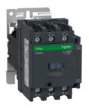
IEC contactor, TeSys D, nonreversing, 65A, 40HP at 480VAC, up to 100kA SCCR, 3 phase, 3 NO, 24VDC coil, open style
