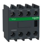
TeSys Deca, auxiliary contact block, 3 NO and 1 NC, top mount, screw clamp terminals, for LC1D09 to LC1D150 contactors
