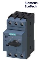
Circuit breaker size S00 for motor protection, CLASS 10 A-release 7...10 A N release 130 A screw terminal Standard switching capacity
