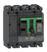
Circuit breaker, ComPacT NSX100B, 25kA/415VAC, 4 poles 4D (neutral fully protected), TMD trip unit 16A
