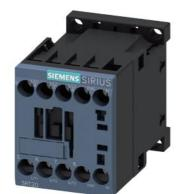
power contactor, AC-3e/AC-3, 7 A, 3 kW / 400 V, 3-pole, 230 V AC, 50/60 Hz, auxiliary contacts: 1 NC, screw terminal, size: S00
